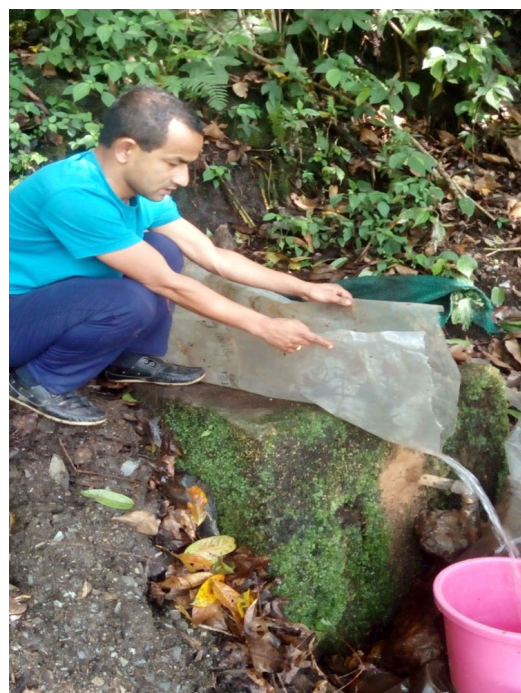
Fig 3: Spring Discharge Measurement in Bikmat
